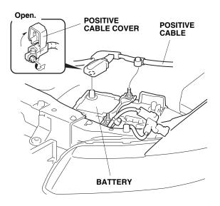
7. Remove the two nuts from the battery setting plate, then remove the battery setting plate and J-bolts. Remove the battery upper cover, the battery, and battery under cover.
