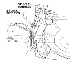
18. Route the heater harness through the front bulkhead as shown. Using one black wire tie, secure the heater harness to the vehicle harness.
