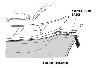
On each side, release five retaining tabs.
