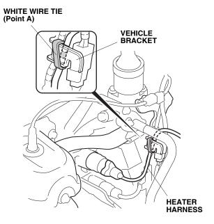
13. Route the heater harness along the fan shroud as shown. Secure the heater harness to the fan shroud rib with one white wire tie at the mark you made (Point B).
